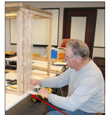
11. Use spacer to get uniform height of stakes on the frame.
